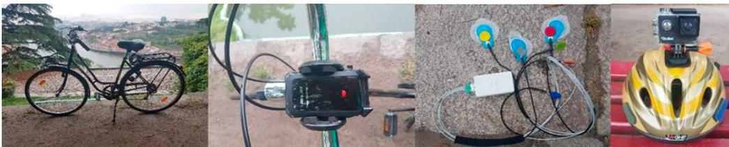
Fig. 2. Tested bicycle; Prototype components (GNSS, HR sensors, and video camera) used for the real time monitoring.
